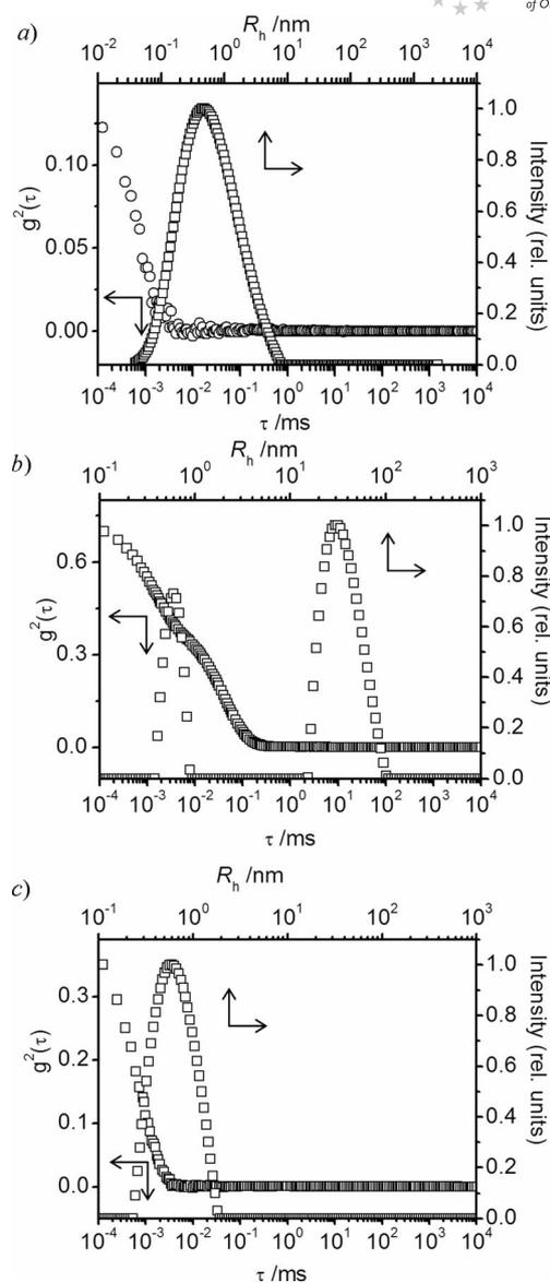
Figure 3. Correlation functions and intensity-weighted size distributions in solution of the glycosyl donor **1b** (a), glycosyl acceptor **5** (b), and their 1:1 mixture (c) in MeCN at 69 mM concentration.
