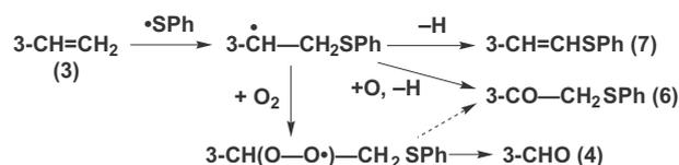
**Scheme 2.** A possible radical mechanism for oxidative cleavage of the C3-vinyl group.
