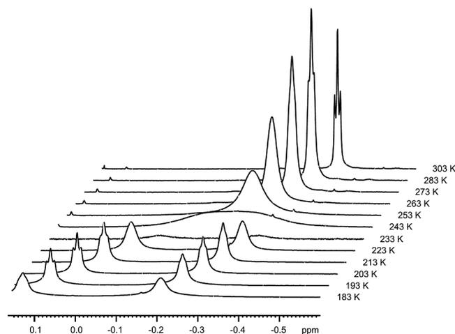
**Figure 4.** Decoalescence of the  $\text{AlMe}_2$  resonance in a variable temperature <sup>1</sup>H NMR spectroscopic investigation of a solution of **5** in  $[\text{D}_8]\text{toluene}$ .
