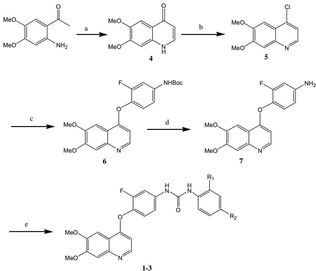
**Scheme 3.** Synthetic routes for the production of VEGFR-2/PDGFR dual inhibitors. Reagents: (a) NaOMe, ethyl formate; (b) oxalyl chloride, DCM; (c) (3-fluoro-4-hydroxy-phenyl)-carbamic acid *tert*-butyl ester, DMF, DMAP; (d) HCl/dioxane; (e) triphosgene followed by a reaction with a corresponding aniline.
