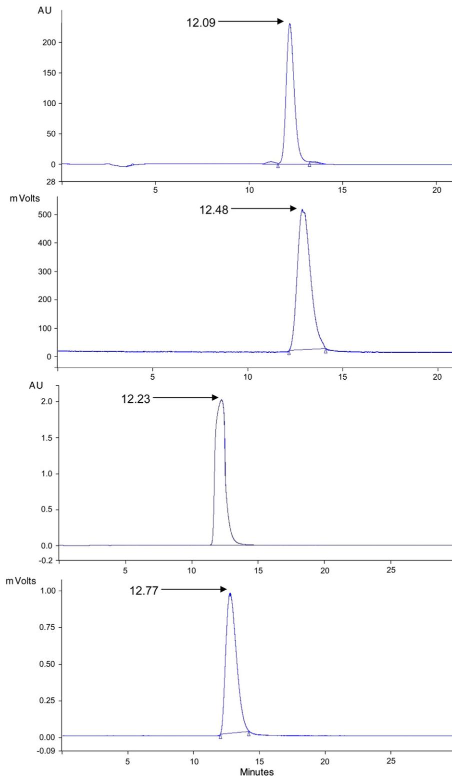
**Figure 1.** HPLC chromatograms of analytical injections of **1**, [ $^{18}\text{F}$ ]-**1** and a co-injection of the two. From top to bottom: UV chromatogram of **1**, Radio chromatogram of [ $^{18}\text{F}$ ]-**1**, A co-injection of **1** and [ $^{18}\text{F}$ ]-**1** showing both UV and radio chromatograms. A difference of  $\sim 0.5$  min exists between the UV and radio peaks since the solvent passes through UV detector and only then through the radioactivity detector.
