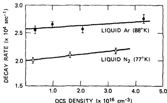
FIG. 3. Decay rate of S(<sup>1</sup>S) vs [OCS] in liquid argon (88 °K) and liquid N<sub>2</sub> (77 °K).
