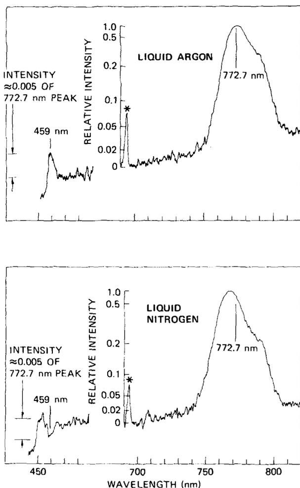
FIG. 1. Emissions following the production of S(<sup>1</sup>S) from OCS photodissociation in the wavelength region 140–161 nm, in both liquid argon (88 °K) and liquid nitrogen (77 °K). OCS = 0.35 ppm. Asterisks indicate scattered light from the H<sub>2</sub> photolysis lamp.
