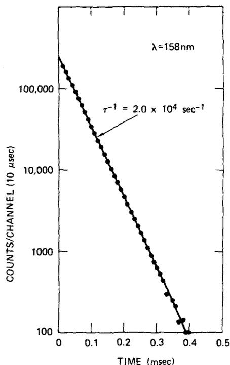
FIG. 2. Decay of S(<sup>1</sup>S) in liquid N<sub>2</sub> (77 °K) containing [OCS] =  $0.27 \times 10^{16}$  cm<sup>-3</sup>. 3 min experiment at  $\lambda = 158$  nm.
