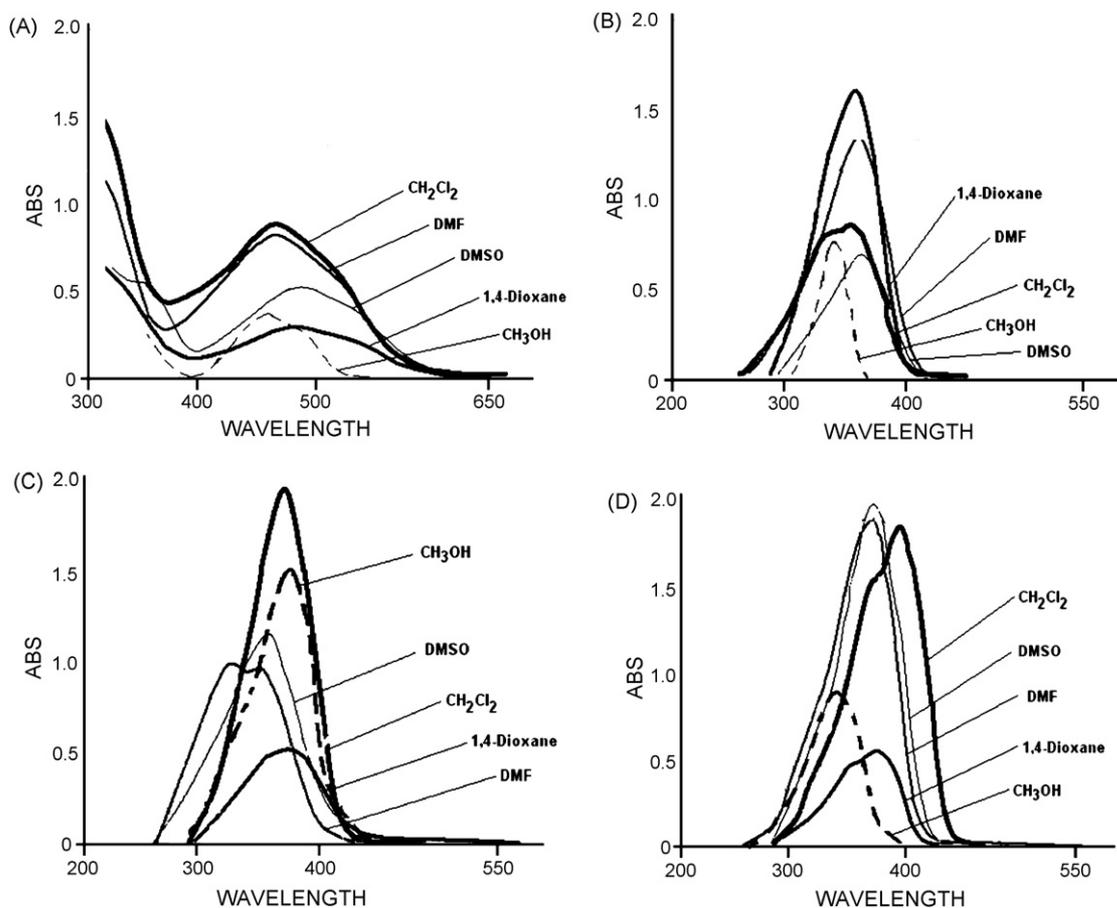
Fig. 5. The electronic absorption in  $\text{CH}_3\text{OH}$ ,  $\text{DMSO}$ ,  $\text{DMF}$ ,  $1,4\text{-Dioxane}$ ,  $\text{CH}_2\text{Cl}_2 \cdot 10^{-4} \text{ mol/l}$ : (A) compound **1**; (B) **2**; (C) **3**; (D) **5**.
