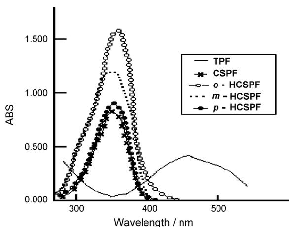
Fig. 4. The electronic absorption of formazans in  $\text{CH}_3\text{OH}$ ,  $10^{-4}$  mol/l.
