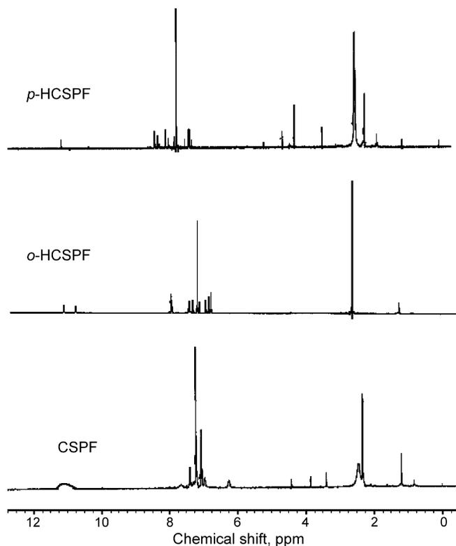
Fig. 1.  $^1\text{H}$  NMR spectra of CSPF, *o*-HCSPF, *p*-HCSPF measured in  $\text{CDCl}_3$  at  $25^\circ\text{C}$ .
