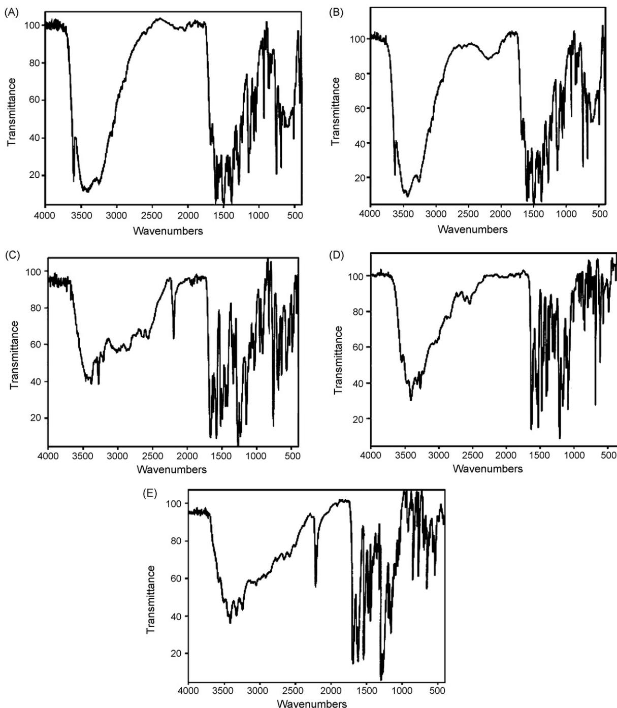
Fig. 2. IR spectra of: (A) TPF; (B) CSPF; (C) *o*-HCSPF; (D) *m*-HCSPF; (E) *p*-HCSPF.
