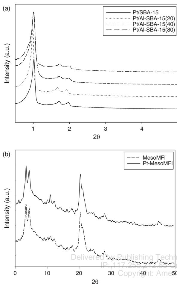
**Fig. 1.** (a) Low angle, and (b) high angle XRD patterns of prepared catalysts.
