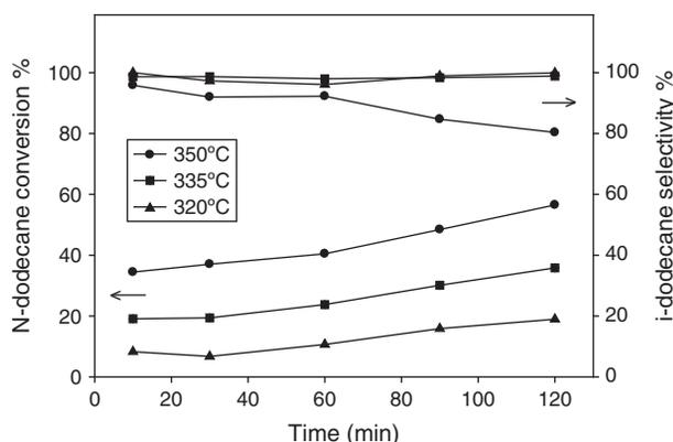
**Fig. 4.** Effect of reaction temperature on *n*-dodecane conversion and isomer selectivity.
