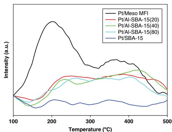
**Fig. 2.** NH<sub>3</sub> TPD of various catalysts.
