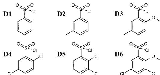
**Figure 5.** The six building blocks selected for the D-pocket.
