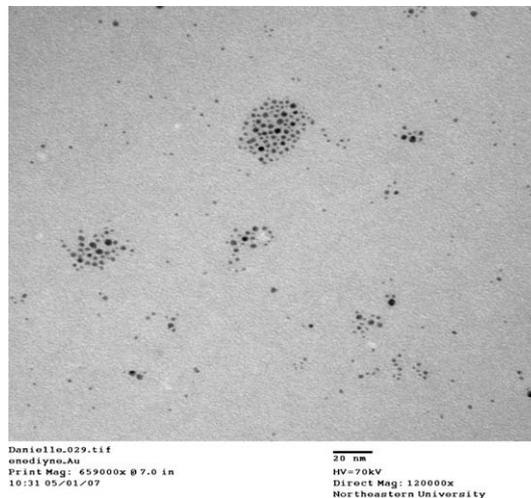
Figure 1. TEM image of Au enediynenanoparticles 27.
