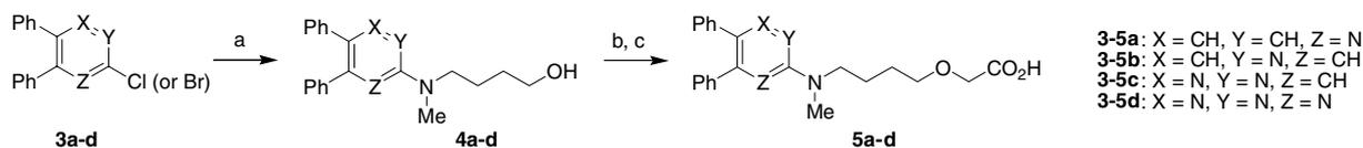
**Scheme 1.** Reagents and conditions for synthesis of **5a–d**: (a) 4-(methylamino)-1-butanol (10 equiv for **3a,b**, and c, 1.5 equiv for **3d**), **3a**, neat, 100 °C; **3b**, neat, 190 °C; **3c**, neat, 170 °C; **3d**, K<sub>2</sub>CO<sub>3</sub>, DMF, rt; (b) BrCH<sub>2</sub>CO<sub>2</sub>*t*-Bu, *n*-Bu<sub>4</sub>NHSO<sub>4</sub>, aq KOH, benzene, 0 °C to rt; (c) 1 N NaOH, MeOH, reflux.
