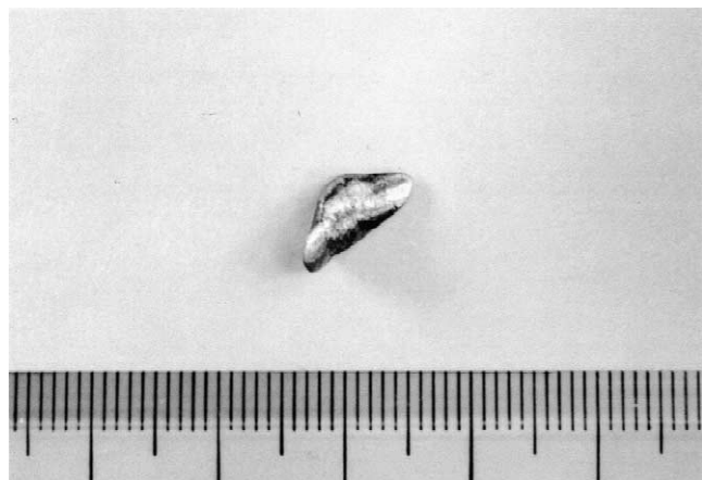
Fig. 3. A 0.876-g sample of cerium metal decomposed at 1250 °C.
