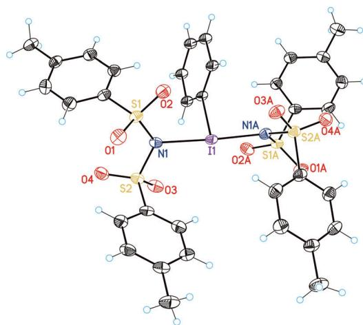
**Figure 1.** X-ray crystal structure of **4**; ellipsoids at 50% probability. Selected bond lengths [ $\text{\AA}$ ] and angles [ $^\circ$ ]: I1–C15 2.117(17), I1–N1 2.210(4), I1–N1A 2.210(4); C15–I1–N1 88.37(10), N1–I1–N1A 176.7 (2).
