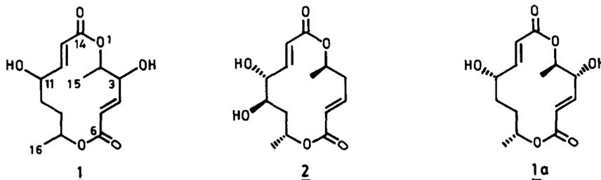
By analogy with colletodiol (**2**) the absolute stereochemistry of **1** at C-2, C-8 and C-11 was assumed to be 2R, 8R and 11S, while the new stereocentre at C-3 could be either R or S. At the first instance a protocol was developed to synthesise the 3R isomer i.e. (2R, 3R, 8R, 11S) **1a** by a convergent approach.
