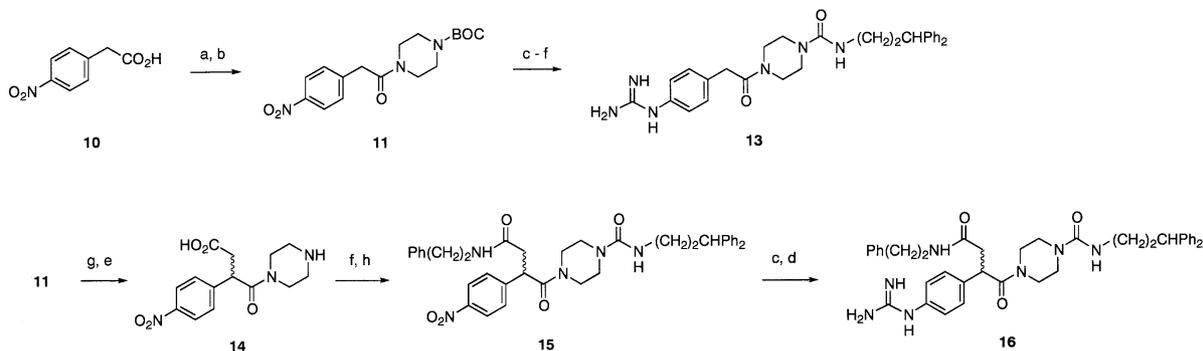
**Scheme 3.** Preparation of 4-(guanidinophenyl)acetyl piperazine derivatives. Reagents and conditions: (a) SOCl<sub>2</sub>, reflux; (b) *tert*-butyl 1-piperazinecarboxylate, DIPEA, THF, -78 °C; (c) 10% Pd/C, H<sub>2</sub>, MeOH; (d) NH<sub>2</sub>CN, 4 N HCl in 1,4-dioxane, 60 °C; (e) TFA; (f) Ph<sub>2</sub>CH(CH<sub>2</sub>)<sub>2</sub>N=C=O (**12**), DIPEA, DMF; (g) NaH, *t*-butyl bromoacetate, 0 °C; (h) Ph(CH<sub>2</sub>)<sub>2</sub>NH<sub>2</sub>, EDC, HOBT, DMF.
