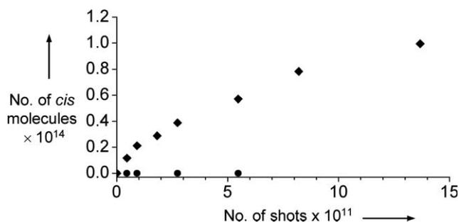
**Fig. 5** Time courses in the photoisomerization of **1**<sub>trans</sub> to **1**<sub>cis</sub> ( $\blacklozenge$ : 1 mL of a rapidly stirred 2.5  $\mu$ M THF solution in a 1 cm cell) and **3** ( $\bullet$ : 0.4  $\mu$ M THF solution) using two-photon excitation with 200 fs pulses at 890 nm. The progress of the isomerization was monitored at 505 nm.
