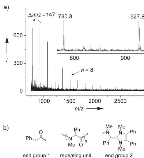
**Figure 1.** MALDI-TOF MS analysis of polypeptides. a) The spectrum of **3a** (Table 1, entry 1) obtained in the reflection mode with 2,5-dihydroxybenzoic acid (DHB) as the matrix. The inset is an expansion of the  $m/z$  region from 770 to 940. b) Tentative assignment of the end group structures.
