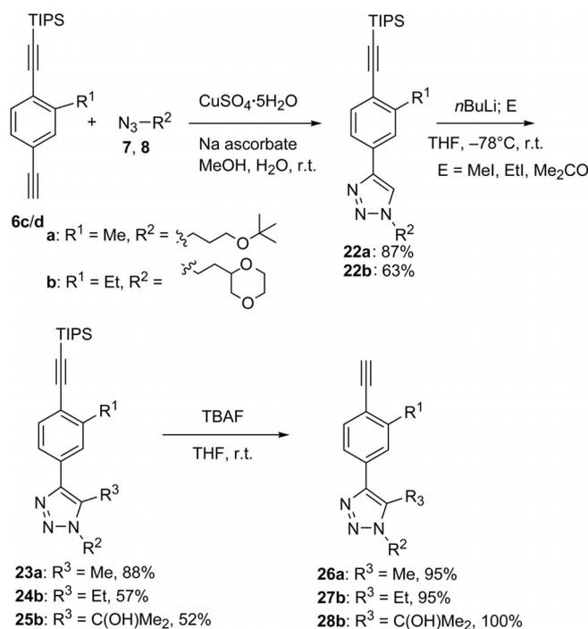
Scheme 6. Synthesis and modification of the bottom ring in the scaffold **B**.
