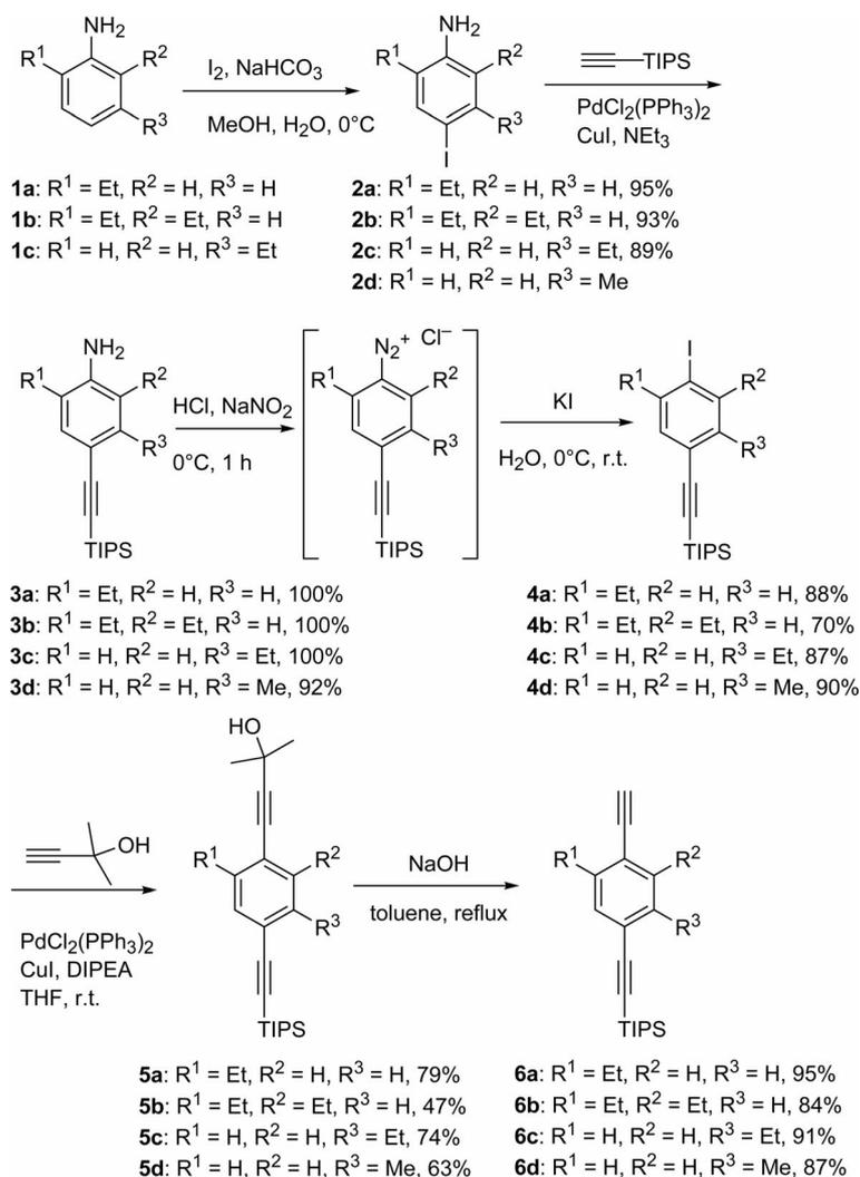
Scheme 2. Synthesis of the 1,4-dialkynylbenzene intermediates **6a–d**. Compound **2d** was purchased.
