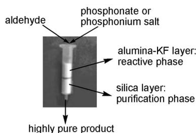
Figure 1. SPE column loaded with a layer of alumina-KF and a layer of silica.
