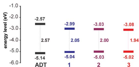
Figure 4 Electrochemically derived HOMO and LUMO energy levels of compounds 1–3 and ADT
