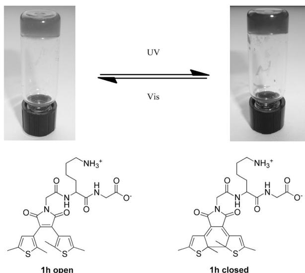
**Figure 6.** Ring closing/opening in a hydrogel of **1h** ( $44 \text{ mg mL}^{-1}$ ) by using irradiation at 312 nm and  $> 500 \text{ nm}$ , respectively.
