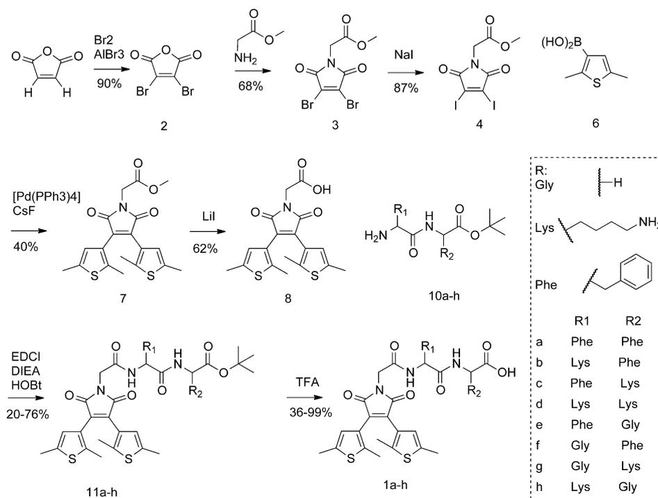
Scheme 1. Synthesis of **1a–1h** (EDCI = 1-ethyl-3-(3-dimethylaminopropyl)carbodiimide, DIEA = *N,N*-diisopropylethylamine, HOBt = 1-hydroxybenzotriazole, TFA = trifluoroacetic acid).
