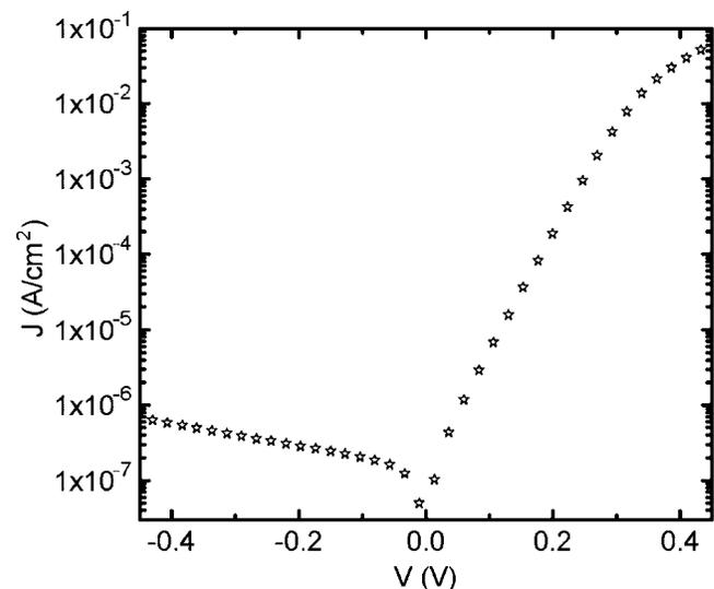
FIG. 3. Current-voltage characteristics from a typical Bi(0001)/GaAs(111) diode grown at  $70^\circ\text{C}$ . The extracted barrier height from the intercept of the  $I$ - $V$  curve was  $\Phi_B^{\text{IV}}=0.77$  eV, with an ideality factor  $n=1.05$ .
