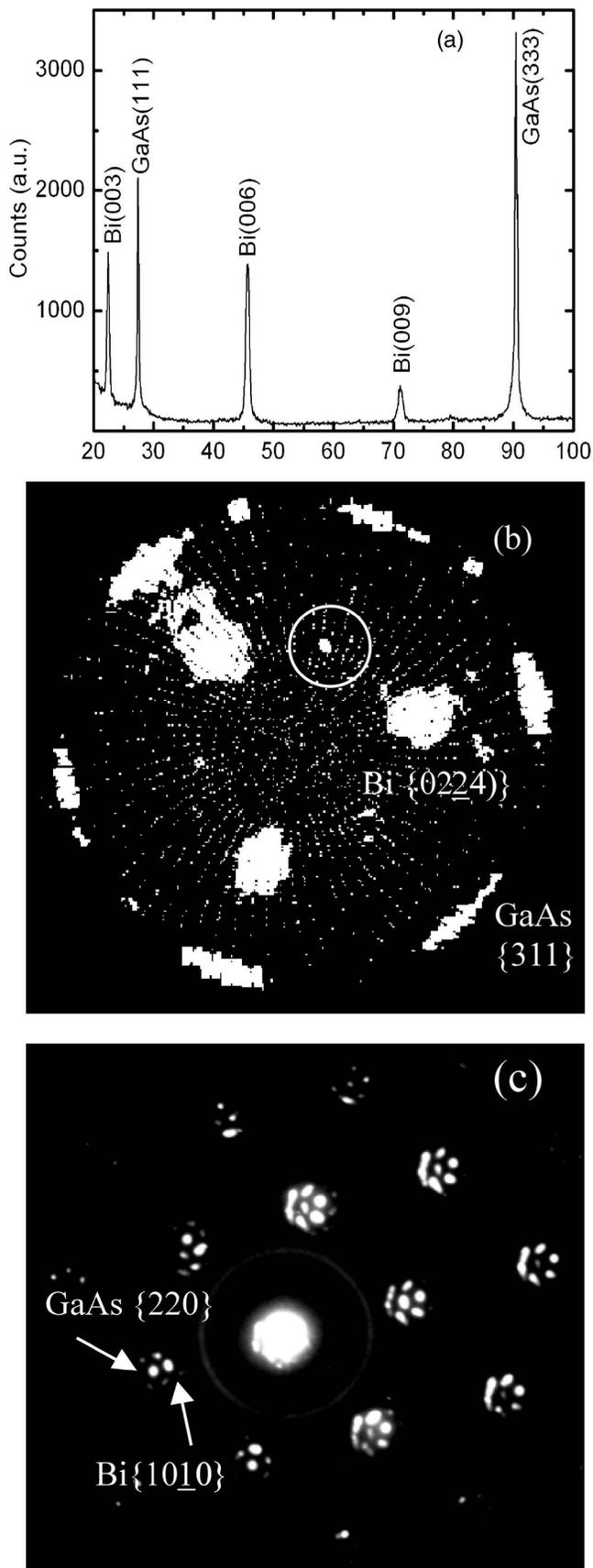
FIG. 1. (a) X-ray diffraction spectra ( $\theta$ - $2\theta$ ) of Bi films electrodeposited from saturated  $\text{Bi}(\text{NO}_3)_3$  and  $(\text{NH}_4)_2\text{SO}_4$  (0.3 M) solutions at  $70^\circ\text{C}$  on GaAs (111); (b) Bi {0224} x-ray pole figure; (c) A plan-view TEM diffraction pattern with the beam normal to the film and substrate surfaces. The extra spots around each of the Bi {1010} and GaAs {220} primary spots are due to double diffraction.
