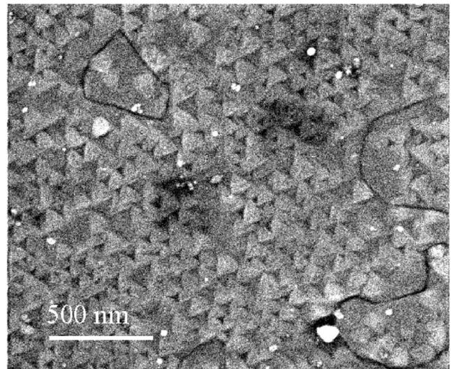
FIG. 2. A secondary electron image from scanning electron microscopy of the surface of a Bi/GaAs (111) film. The triangle shapes indicate the development of a threefold symmetric surface facet consistent with single crystalline Bi. Also visible are rotation boundaries due to twinning.
