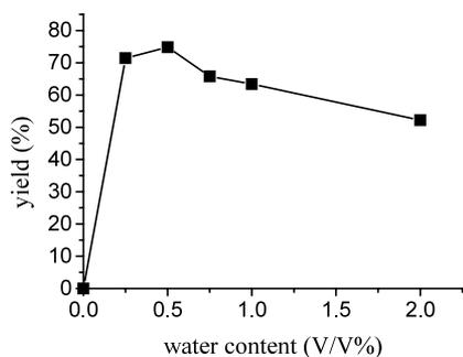
**Figure 1.** The effect of water content on the yield of Z-PheGlyGlyOEt catalyzed by  $\alpha$ -chymotrypsin in cyclohexane.
