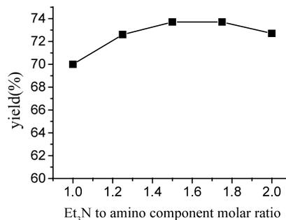
**Figure 2.** The effect of the amount of  $\text{Et}_3\text{N}$  on the yield of Z-PheGlyGlyOEt catalyzed by  $\alpha$ -chymotrypsin in cyclohexane.
