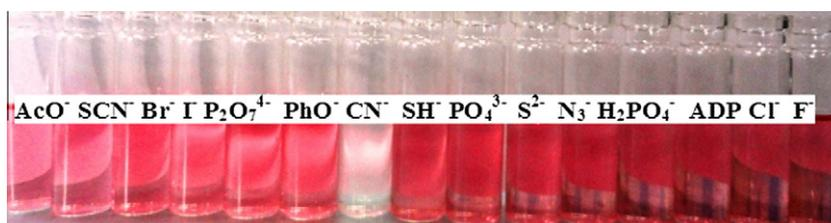
**Figure 2.** Visual changes of TBH ( $c = 2.0 \times 10^{-6}$  M) with addition of 1.0 equiv of each anion ( $c = 2.0 \times 10^{-5}$  M) at pH 7.1 in  $\text{CH}_3\text{CN}/\text{H}_2\text{O}$  (1:1, V/V).
