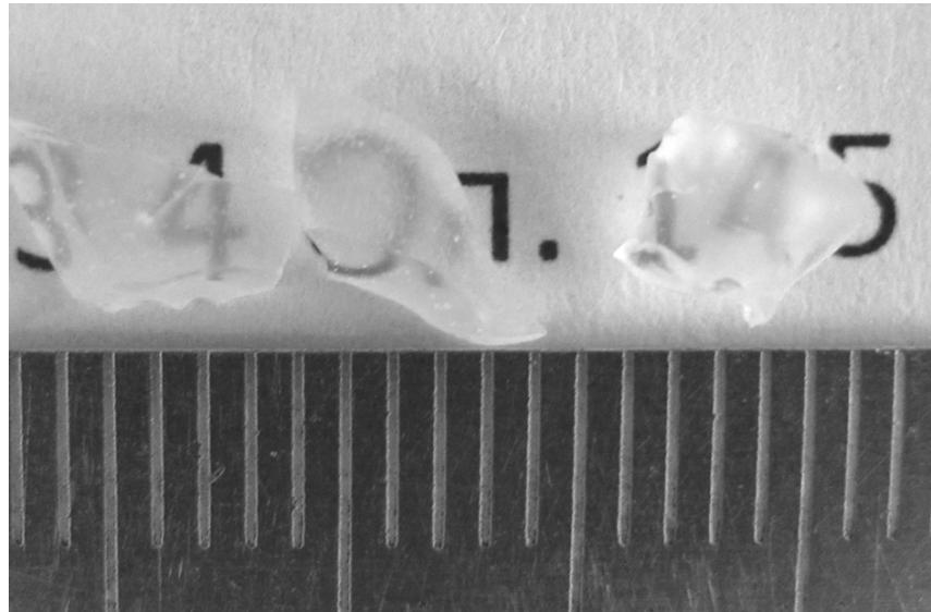
**Fig. 4.** Photographs of translucent xerogels used as precursors to magnesium aluminum spinel. The mean sample thickness is 2.3 mm.
