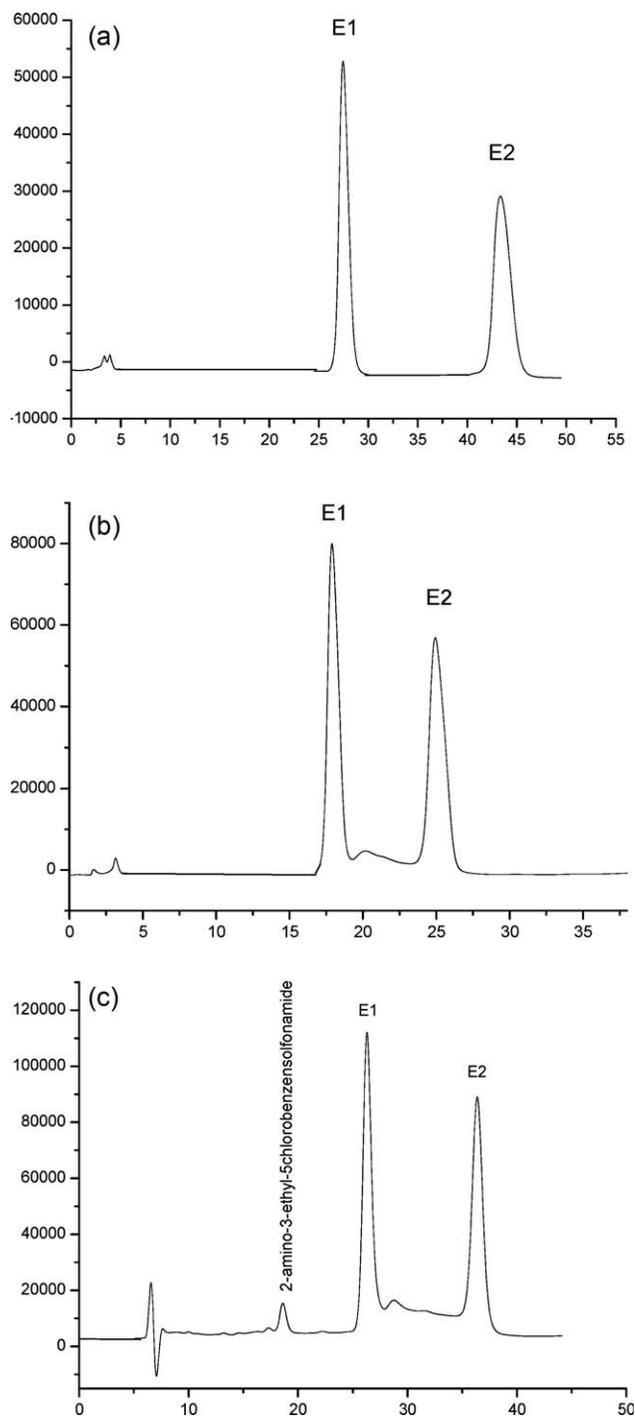
**Fig. 3.** On-column enantiomerization and hydrolysis of ( $\pm$ )-**1**; flow rate: 0.5 ml/min, Column: Chiralcel OD-RH (150 mm  $\times$  4.6 mm I.D.; 5  $\mu\text{m}$ ); (a) water:acetonitrile 60:40 (v/v);  $T = 0^\circ\text{C}$ , (b) water:acetonitrile 60:40 (v/v);  $T = 37^\circ\text{C}$ , (c) buffer pH 2.20 (0.05 M  $\text{NaClO}_4/\text{HClO}_4$ ): acetonitrile 60:40 (v/v);  $T = 37^\circ\text{C}$ .
