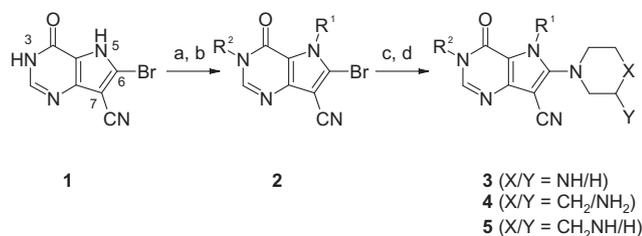
**Scheme 1.** Synthesis of 7-cyanodeazahypoxanthines. (a) R<sup>1</sup>X, DIPEA, DMF, rt, 18 h. (30–69%); (b) R<sup>2</sup>X, K<sub>2</sub>CO<sub>3</sub>, DMF, rt, 1 h, (63–97%); (c), Boc diamine, DMA,  $\mu$ -wave, 160 °C, 45 min (40–90%); (d) TFA/DCM [1:1], rt, 1 h, (70–95%).
