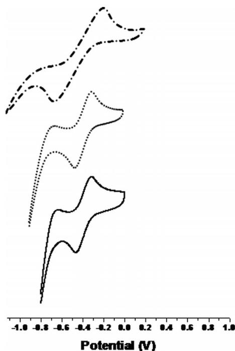
Figure 4. Cyclic voltammograms of **5** (—), **4** (···) and **7** (-·-·-) in  $\text{CHCl}_3$ .
