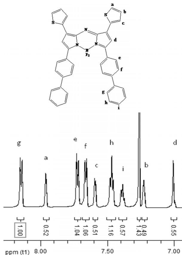
Figure 1.  $^1\text{H}$  NMR spectrum of **1** recorded in  $\text{CDCl}_3$ .
