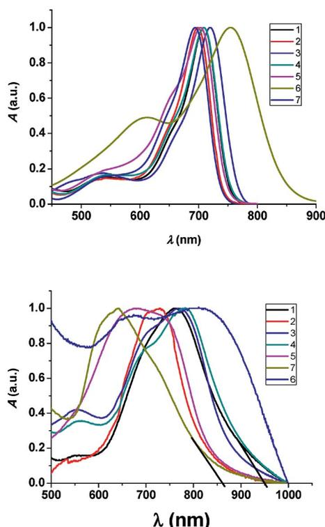
Figure 2. Normalized absorption spectra for **1–7** in  $\text{CHCl}_3$  (top) and in thin films (bottom).
