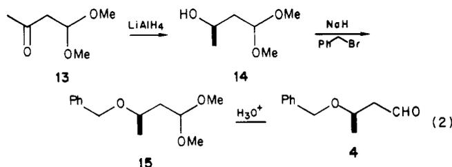
13 provides alcohol 14. Benzoylation of this material gives 15, which is hydrolyzed to obtain 4.
