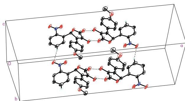
**Fig. 2** Part of the crystal structure of (I), showing the formation of a hydrogen bonded dimer and  $R_4^4$  motif built from paired O–H…O and C–H…O hydrogen bonds (dashed lines). For the sake of clarity, the H atoms not involved in the hydrogen bonds have been omitted
