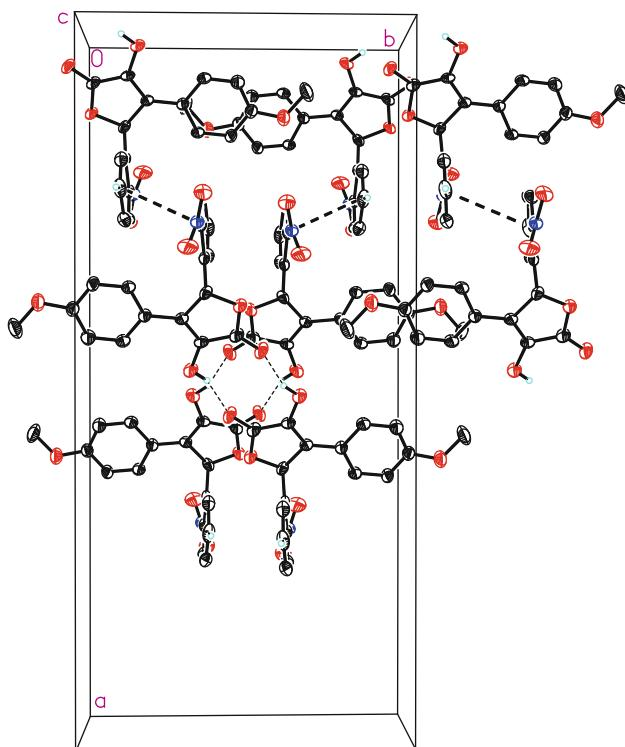
**Fig. 4** Packing diagram of compound (I) viewing along c-axis, Solid dashed lines indicate  $\pi$ – $\pi$  interactions
