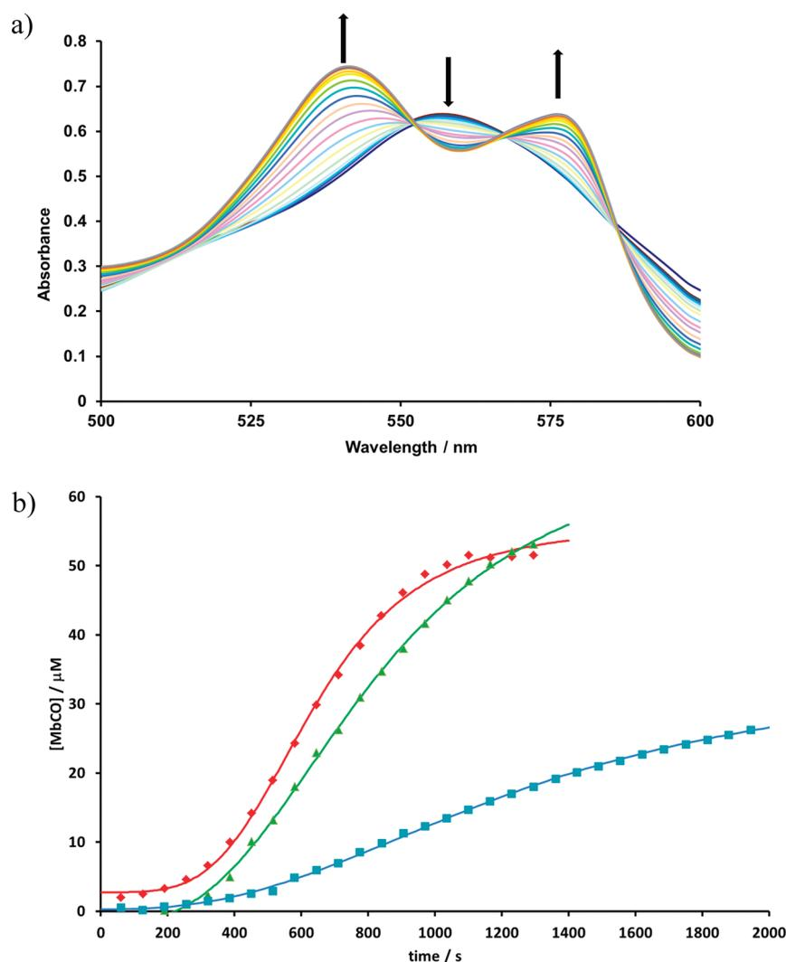
**Figure 7.** CO release profile for **1**. (a) UV–vis spectrum showing the Q-bands during the conversion of deoxy-Mb to MbCO with time for a 60  $\mu\text{M}$  solution. (b) Plot of [Mb-CO] against time: (red  $\blacklozenge$ ) [1] = 60  $\mu\text{M}$ , (green  $\blacktriangle$ ) [1] = 40  $\mu\text{M}$ , and (blue  $\blacksquare$ ) [1] = 20  $\mu\text{M}$ .
