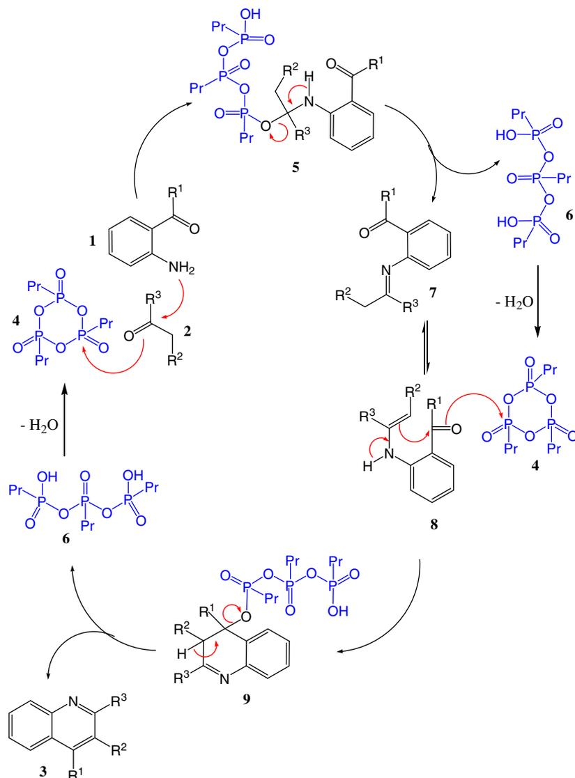
Scheme 1. Proposed mechanism of the T3P catalyzed quinoline synthesis.
