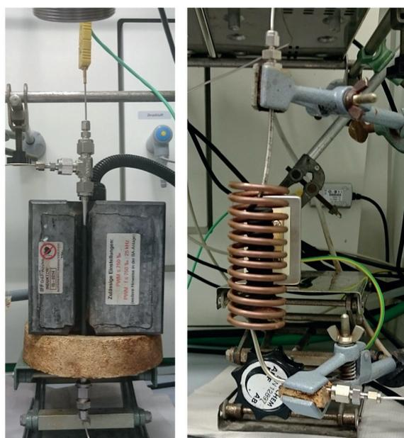
**Figure 2.** Temperature versus power input for a 1/4" steel reactor at 15.0 kHz; the temperature was measured at the outlet of the reactor using the K-element (top); 1/4" steel reactor encased in middle frequency inductor (bottom left); 1/8" coil reactor encased in high frequency inductor (bottom right).
