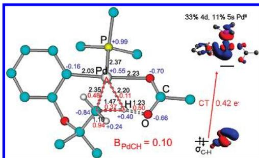
**Figure 1.** Calculated TS for concerted palladation–deprotonation. Select H atoms have been removed for clarity. Relevant two- and three-center bond orders (red), distances (Å) (black), and NPA-derived atomic charges (blue) are shown. The three-center covalent interaction and charge transferred (CT) from the C–H bond to the metal-based acceptor orbital are shown at right.<sup>13</sup>
