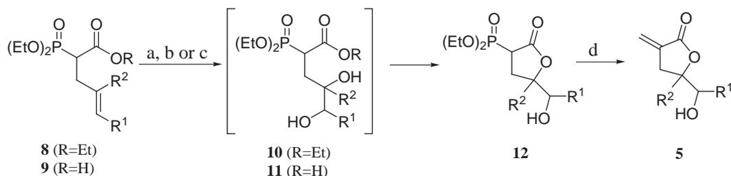
**Scheme 2.** Conditions: (a) OsO<sub>4</sub> cat., NMO, H<sub>2</sub>O/acetone, rt, 24 h; (b) MCPBA, CH<sub>2</sub>Cl<sub>2</sub>, rt, 24 h then 30% HClO<sub>4</sub>, rt, 24 h; (c) AD-mix- $\alpha$  or AD-mix- $\beta$ , 50% aqueous *tert*-BuOH, 0°C to rt, 48 h; (d) 36% formalin, K<sub>2</sub>CO<sub>3</sub>, 0–5°C, 15 min.
