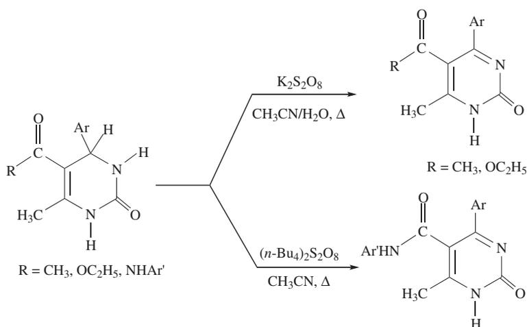
**Scheme 1:** Thermal oxidation of 2-oxo-1,3,4-tetrahydropyrimidines.
