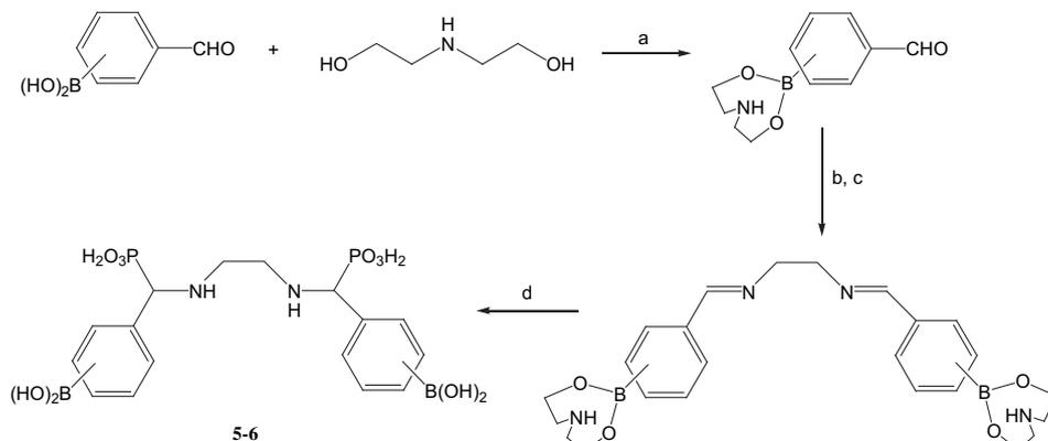
**Fig. 3.** Synthesis of *N,N*-ethyl aminoboronbenzylphosphonates **5–6**. a) THF, 2-propanol, b) ethylenediamine, MeOH, c) DCM,  $P(OSiCH_3)_3$ , d) 10% MeOH in  $H_2O$ .
