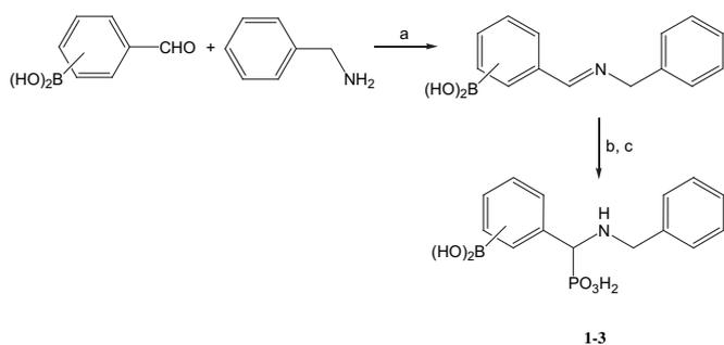
**Fig. 1.** Synthesis of aminoboronbenzylphosphonates **1–3**. a) DCM (using Dean–Stark adapter), b) DCM,  $P(OSiCH_3)_3$ , c) 10% MeOH in  $H_2O$ .
