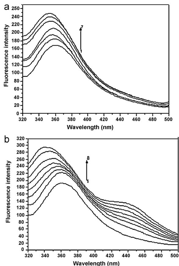
Fig. 2. Fluorescence emission spectra of  $1.0 \times 10^{-6}$  mol/L Wogonin in CDs. (A):  $\beta$ -CD; (B): HP- $\beta$ -CD. CD concentration (M):  $\beta$ -CD:  $0$ – $6.0 \times 10^{-3}$ ; and HP- $\beta$ -CD:  $0$ – $7.0 \times 10^{-3}$ .
