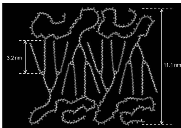
**Fig. 7** Interdigitated lamellar model of **2G-2400**.
