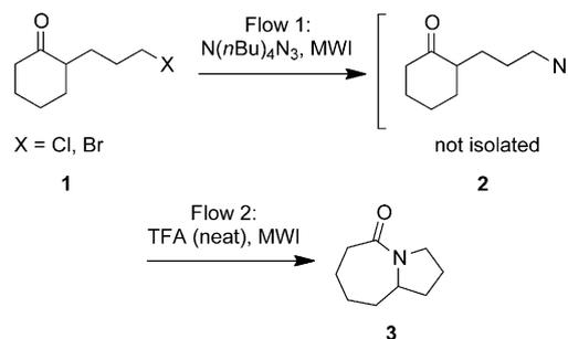
Scheme 1. General reaction sequence. (MWI = microwave irradiation)
