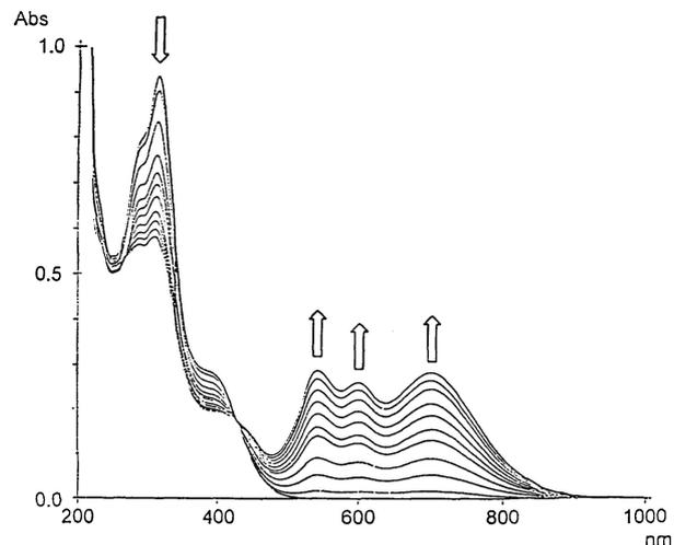
**Figure 2.** Continuous changes in the UV–vis spectra of **1** upon constant-current electrochemical oxidation (29  $\mu A$ ) at 2 min intervals in MeCN.
