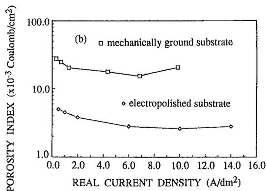
Fig. 2. Nickel porosity as a function of real plating current density on either mechanically ground or electropolished bronze (Watts bath, 55°C, pH 3.4, nickel thickness 0.2  $\mu\text{m}$ ).
