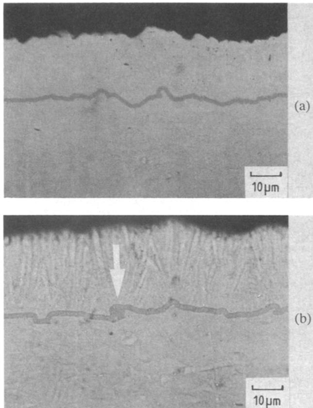
Fig. 5. Cross section of nickel coatings (Watts bath, 55°C, pH 3.4) on mechanically ground bronze: (a) uniform coating thickness, nominal plating current density 6 A/dm<sup>2</sup> (i/i<sub>L</sub>: 0.27) and (b) an area of somewhat thicker coating, nominal plating current density 14 A/dm<sup>2</sup> (i/i<sub>L</sub>: 0.62).
