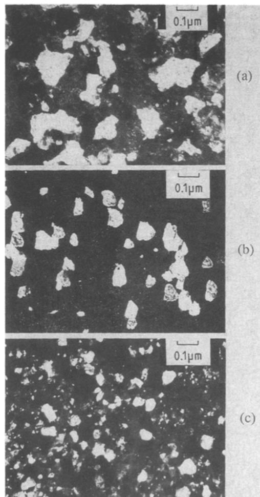
Fig. 3. Dark field transmission electron micrographs of the Watts nickel coatings (55°C, pH 3.4, nickel thickness: 0.2  $\mu\text{m}$ ): (a) real plating current density 0.5  $\text{A}/\text{dm}^2$ , overpotential 508 mV; (b) real plating current density 6  $\text{A}/\text{dm}^2$ , overpotential 1123 mV; and (c) real plating current density 14  $\text{A}/\text{dm}^2$ , overpotential 1860 mV.
