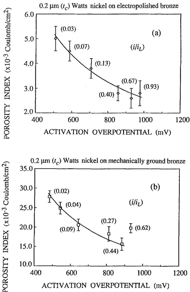
Fig. 4. Porosity index of 0.2 μm thick Watts nickel coatings vs. activation overpotential in plating: (a) on electropolished bronze and (b) on mechanically ground bronze.
