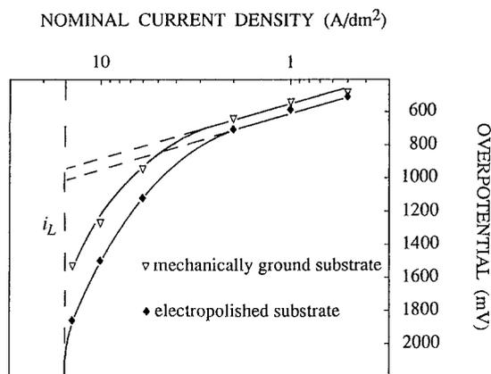
Fig. 1. Polarization for Watts nickel plating (55°C, pH 3.4) on either a mechanically ground or an electropolished substrate.
