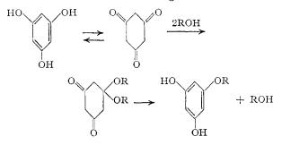
Our method of preparation of the mono-ethers consisted in dissolving anhydrous phloroglucinol and two moles of the alcohol in anhydrous dioxane; the solution was then cooled in an ice-bath, saturated with hydrogen chloride, and kept in the dark at room temperature for a period of one to two weeks.
