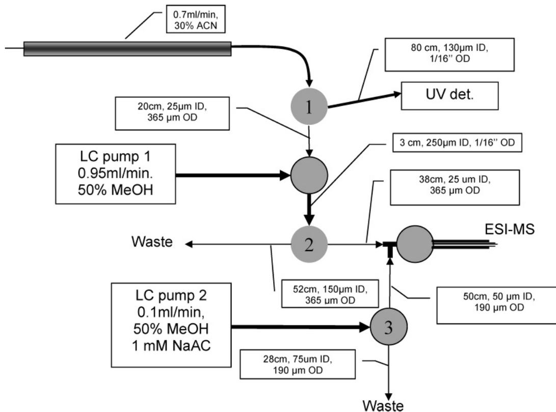
**Figure 1.** Illustration of the flow-splits and the makeup flows between the column and the mass spectrometer. Flow-split: (1) splits the flow 1:350 times, (2) 1:950 times, and (3) 1:10 times.
