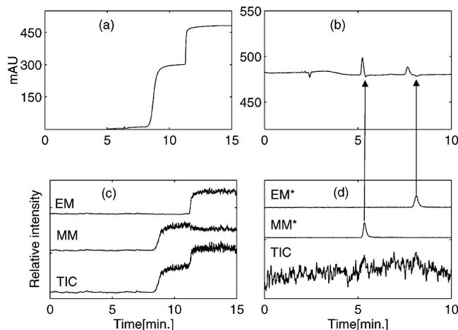
**Figure 4.** Parts a and c show the breakthrough of the eluent 40/40 mM of MM/EM and parts b and d show the elution of a 20  $\mu$ L injection of 7.5/7.5/50/50 mM of MM\*/EM\*/MM/EM on a concentration plateau of 40/40 mM of MM/EM. The top row (a, b) is the UV-detector signal, and the bottom row (c, d) shows the MS signals. Observe that the MS baselines have been moved for easier visualization. TIC is the total ion count.
