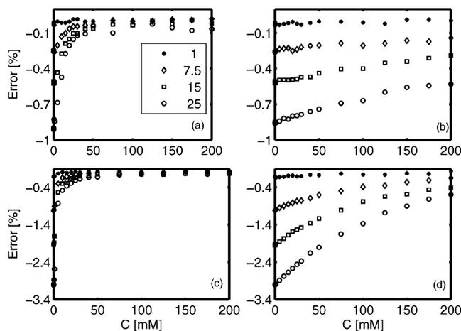
**Figure 2.** The relative error in the retention time versus eluent concentration for the tracer peak (a, c) and the perturbation peak (b, d), respectively, calculated for a 20  $\mu\text{L}$  injection of 1, 7.5, 15, and 25 mM excesses (see legend). Two different Langmuir adsorption isotherms were used (a, b)  $a = 4.59$  and  $b = 2.31 \text{ M}^{-1}$  and (c, d)  $a = 4.59$  and  $b = 9.17 \text{ M}^{-1}$ . The number of theoretical plates was 7030.
