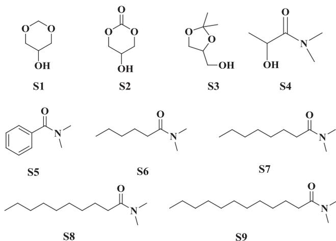
**Fig. 1.** Structures of bio-solvents derived from glycerol (**S1–S3**) and dimethylamide (**S4–S9**) employed in transglycosylation reactions with Biolacta  $\beta$ -galactosidase.
