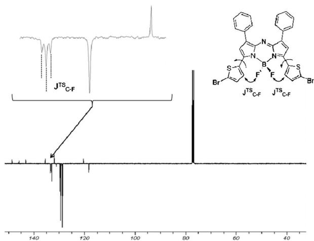
Fig. 2 JMOD  $^{13}\text{C}$  NMR (125.75 MHz,  $\text{CDCl}_3$ ) of **3**.
