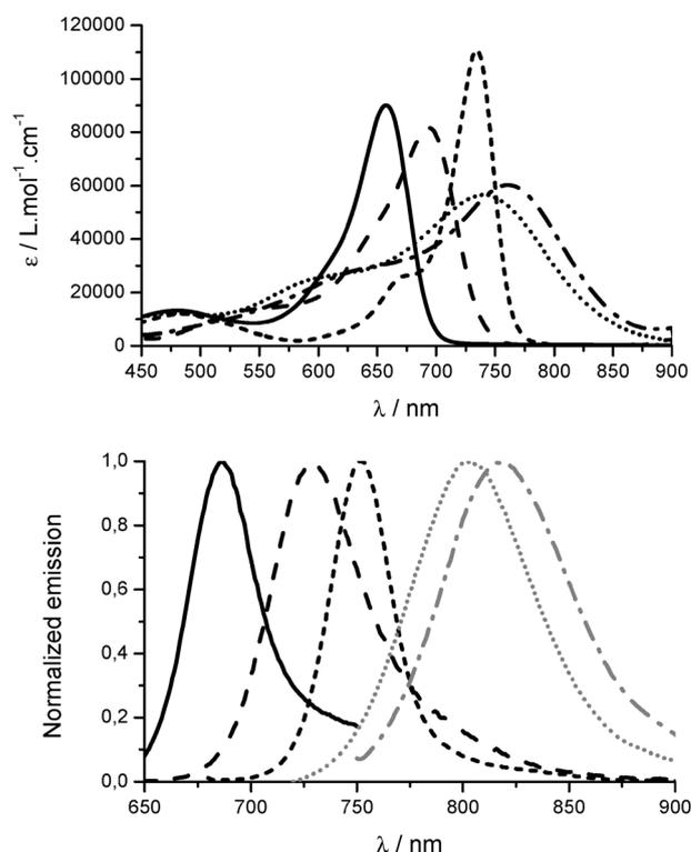
Fig. 3 Absorption (up) and emission (bottom) spectra of **1** (—), **3** (---), **4** (-·-), **5** (···) and **6** (- - -) in dichloromethane (black) and toluene (grey) solution.
