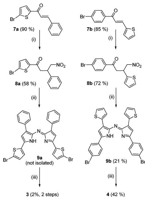
**Scheme 1** Synthesis of the target compounds **3** and **4**. (i)  $\text{CH}_3\text{NO}_2$ ,  $\text{HNET}_2$ , MeOH, reflux; (ii)  $\text{NH}_4\text{OAc}$ , dry BuOH, reflux; (iii)  $\text{BF}_3 \cdot \text{Et}_2\text{O}$ ,  $i\text{Pr}_2\text{EtN}$ , dry  $\text{CH}_2\text{Cl}_2$ , RT.
