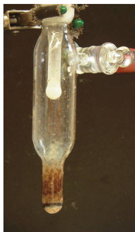
Fig. 4. Sublimation of trans -stilbene from the ionophilic catalyst 8 – [P 66614 ][Cl] reaction mixture using the specially designed reaction tube.
