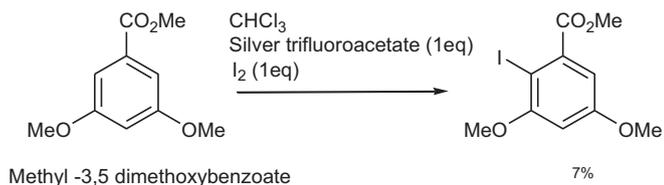
Fig. 4. Preparation of iodo benzo-precursor.
