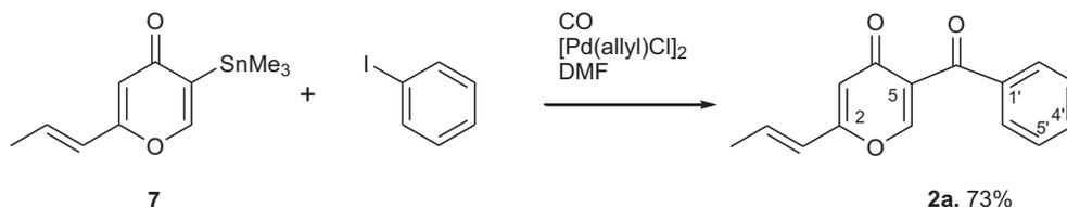
Fig. 5. Coupling reaction between the stannane intermediate **7** and unfunctionalized aryl iodide.
