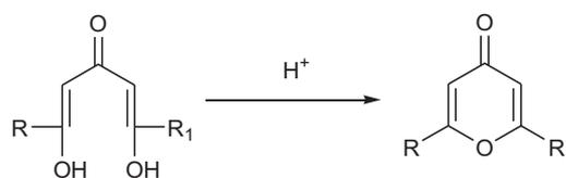
Fig. 2. General synthetic procedures for  $\gamma$ -pyrones preparation.
