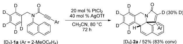
**Scheme 4.** Platinum-catalyzed reaction of [ $\text{D}_5$ ]-**1a**.
