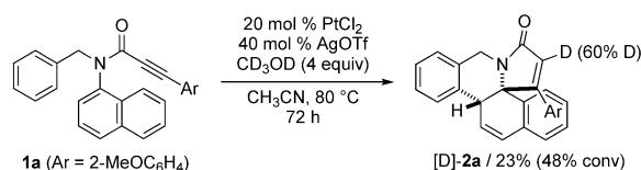
**Scheme 5.** Platinum-catalyzed reaction of **1a** in the presence of  $\text{CD}_3\text{OD}$ .
