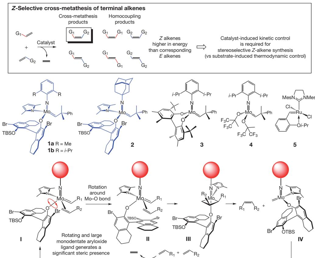
**Figure 1** | A catalytic CM reaction can afford as many as six alkenes, so the challenge is designing an efficient process that favours formation of the cross products. Particularly difficult is the development of a process that affords the higher-energy Z alkene predominantly. To accomplish a Z-selective CM, a variety of catalysts were considered, such as stereogenic-at-Mo complexes (**1**, **2**) or other previously reported Mo- and Ru-based complexes
