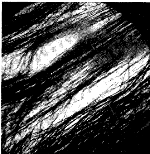
FIG. 1. Ni powder prepared by reduction of aqueous \text{NiSO}_4\text{--NH}_3\text{--}(\text{NH}_4)_2\text{SO}_4 solution with \text{NaH}_2\text{PO}_2 in a 1200-oersted magnetic field. Magnification = 75X.
